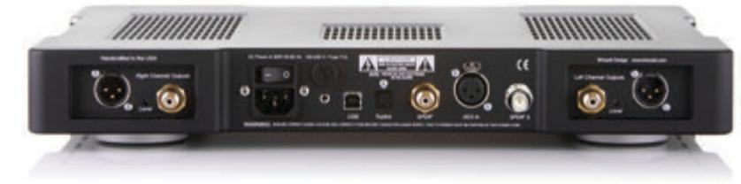
Photo 2: The M1 rear panel features five digital input connections, including USB, AES/EBU, Toslink optical, and S/PDIF via both RCA, and true 75  $\Omega$  BNC connectors. Balanced and unbalanced analog outputs are included. The spacing of the analog outputs reflects the dual-mono design. (Photo courtesy of Bricasti Design, Ltd.)
