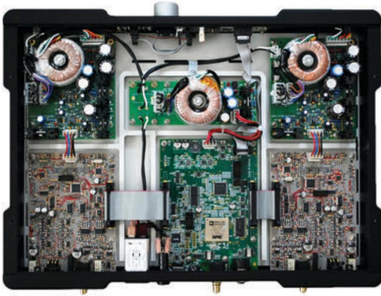
Photo 3: Inside view of the M1 DAC. The dual-mono design includes separate linear power supplies for the left and the right channel audio boards, shown on either side. The linear digital power supply and digital PC board are in the center. Construction is robust, with all chassis pieces machined out of solid blocks of aluminum. (Photo courtesy of Bricasti Design, Ltd.)
